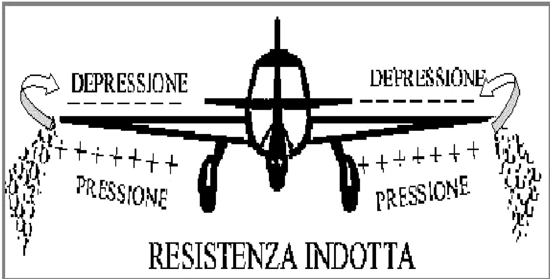
**RESISTENZA DI PROFILO + RESISTENZA INDOTTA = RESISTENZA TOTALE**
